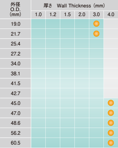
溶接チタン管製造可能範囲 Size Availability of Welded Titanium Pipes and Tubes
